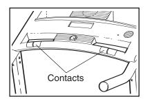
To measure your heart rate, stand on the foot rails. Hold the contacts for approximately 10 seconds—avoid moving your hands. When your pulse is detected, your heart rate will be shown. For the most accurate heart rate reading, continue to hold the contacts for about 15 seconds.
